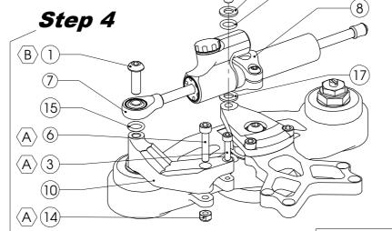
MK-H010-T006 / Honda CBR1000RR 2008 POS **ITEM** SIZE QTY Bolt\_DIN7380 M8x25 B Bolt\_DIN7380 2 M8x55 B 3 Bolt\_DIN912 M5x20 4 4 Bolt DIN912 M6x16 5 Bolt DIN912 M6x25 6 Bolt DIN912 M6x30 7 CSC\_RSC damper S075 8 MP-DB018235 9 MP-ELEC01 MP-FOMK73 10 MP-TAMK63-1 11 12 MP-TAMK63-2 assy MP-TAMK63-3 & -4 13 14 Nut DIN985 M6 3 10.3x2.4 15 O-ring 16 M6\_12\_h1.6 2 Washer 17 M8 16 h1.6 Washer
