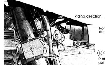
Rotate head lamp rubber so the flaps do not touch the damper
