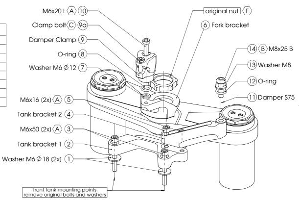
(\*) TORQUES A: 5-9Nm / 44-80Lbs.ln / 4.0-6.4Lbs.Ft B: 14-17Nm / 124-150Lbs.ln / 10.3-12.5Lbs.Ft C: 6Nm / 53Lbs.ln / 4.4Lbs.Ft
