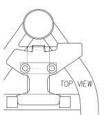
Remove the fake tank cap, the top of the air filter box and the instrument panel from the top of the frame. Place the tank bracket assembly correctly on top of the frame. The front notch has to be placed in the hole behind the steering head. The rear part of the tank bracket has to be placed between the 2 mounting points of the instrument panel. Use the 2 M8x60 countersunk bolts (4) and the steel strip (5) to clamp the tank bracket assembly to the central frame tube.
