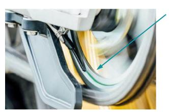
**4.** Scottoil is dispensed onto the face of the rear sprocket where it transfers directly into the chain for perfect lubrication
